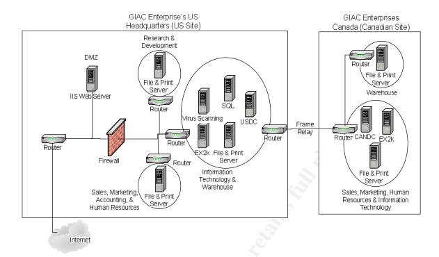
In the proposed diagram there are two domain controller servers, five file and print servers, two Exchange 2000 servers, one Internet Information Server, one SMTP virus scanning server and one SQL server. Each server will be installed with Windows 2000 and have a specific role within the physical site. There are 5 physical sites (three in the US and 2 in Canada) and 2 logical sites, one in the US and one in Canada.
