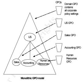
This diagram represents a portion of GIAC Enterprises GPO design, modeled after Microsoft's Monolithic design model.
