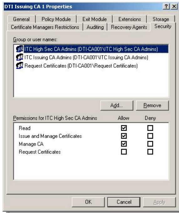
Figure 3-12: The permissions set by the CA administrators on the issuing CAs. The groups are local groups on each CA to which domain global groups have been added.
