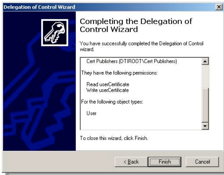
Figure 3-14: Final page of the Delegation of Control Wizard used in giving the Cert Publishers group read and write permissions to the userCertificate attribute on accounts in the DTL.DTIROOT.NET child domain.
