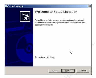
2. Create a new installation file. This file that's created will be the unattended installation script that will be used to automate the operating system installation.
