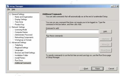
24. Once all of the above configurations have been specified the unattended installation script must be saved to the hard drive to be used later during an actual Windows Server installation.
