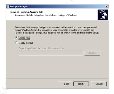
3. Choose to create an unattended installation script. Although a syspreped image could be created here, since this document describes the first terminal server in a farm to be created, sysprep images will be unavailable. Also, since ACME has a limited installation of Microsoft Active Directory which is currently being rolled out to all of the local systems, the Remote Installation Services (RIS) script will not be chosen (since it requires Active Directory to utilize).
