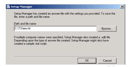
25. This completes the unattended installation script setup process using the Setup Manager utility that comes with Windows Server 2003.
