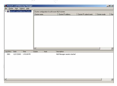
Once the tool is opened, the only process required is to right-click on the node for "Network Load Balanced Cluster" in the left-hand windows and choose "New Cluster" to open the Cluster Manager wizard. The first screen, shown below, prompts the administrator to choose an IP address for the virtual cluster and a name for the cluster. This should not be the IP address of one of the servers that will be a part of the TS
