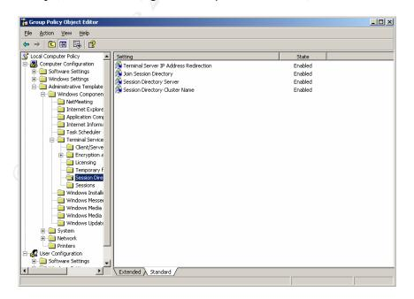
Not only must all of the settings be set to "Enabled," but two of them must be specifically configured to instruct the server as to which server is hosting the TSSD service and what the name of the TSSD cluster is (configured earlier through NLB). The following screens demonstrate the simple configuration of this service through the two GPO settings, "Session Directory Server" and "Session Directory Cluster Name."
