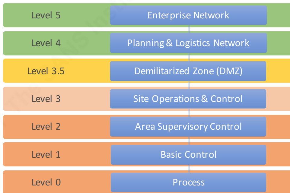
Figure 1 Purdue Enterprise Reference Architecture (PERA) Model
