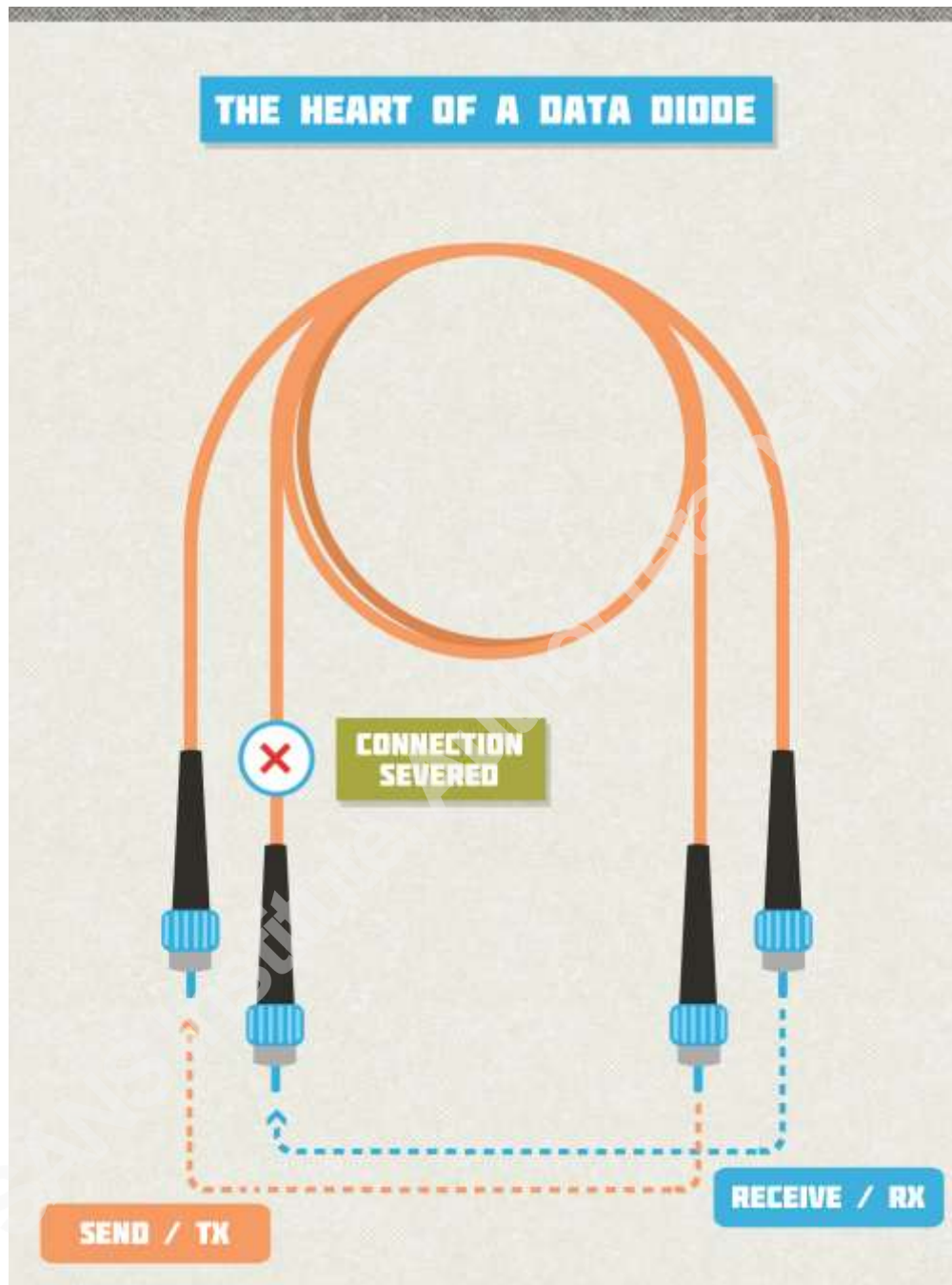
Figure 1 - Base Concept of a Data Diode.
