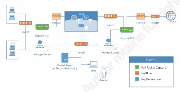
In this example, if both TAPs are not in place, it would complicate the job of an analyst. If the first firewall is providing Network Address Translation (NAT), the analyst would only see one IP address. With both TAPs in place, it offers the full story by showing the internal and public traffic. Thus, allowing an analyst to follow an incident from start to finish.
