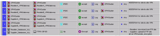
These are the site-to-site VPN rules for the Supplier/Reseller <-> GIAC network to allow encrypted packets between those sites and the GIAC network. Note that in order to actually build the tunnel, shared secrets must be exchanged prior to trying to use the tunnel. Rule 10 then uses the actual tunnel, allowing FTP across to the FTP server, encrypted.
