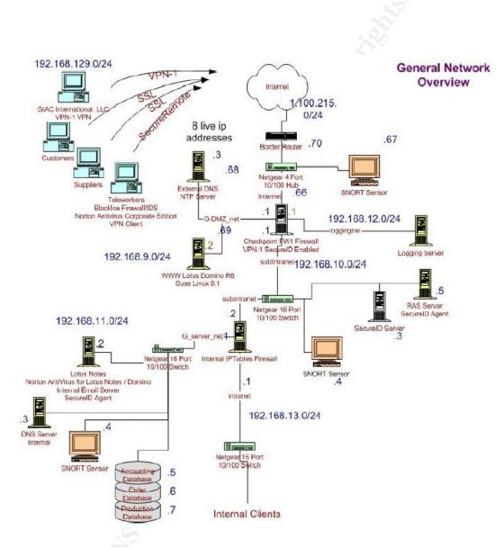
The design uses a Check Point firewall protecting the DMZ and an Internal IPTables firewall protecting critical internal network resources.
