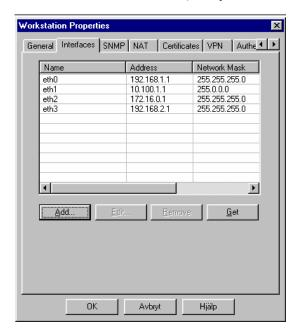
Then you need to modify the Security Property on all interfaces. Be sure to remember to change tracking from "None" to "Log", otherwise you will have a bad time trying to figure out why packets are rejected (and it is very good to know if someone tries a spoofing attack on you). Shown below is the Properties of the Presentation Network:
