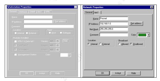
Above, to the left, a workstation object is defined. If it was a firewall, the "VPN -1 & FireWall-1" checkbox would be filled in the "Mo dules Installed" section. To the right, a network object is defined. It is possible to do automatic address translation from the objects, but it gives you fewer options as how to set it up. It also adds to the locations to check for problems when something is amiss. I prefer to keep all NAT in one place.
