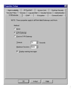
It is up to the administrator to decide which (if any) option is to be used. The SYN Gateway intercepts incoming SYN packets, sends back SYN -ACK and wait for the final ACK. If there is none, Firewall-1 drops the whole connection and the server behind the firewall will never notice the exchange. This could lead to false positives for potential intruders who use SYN scans to map the network because they will get an answer no matter if the host on the other side is up or not.
