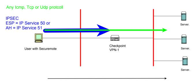
User tunneling traffic to the Secure Domain within at IPSEC Tunne
