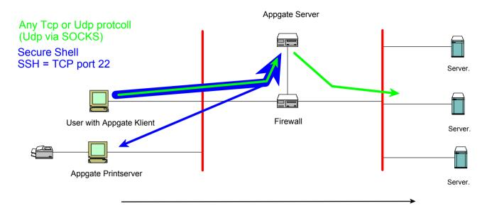
User tunneling traffic to the Secure Domain within at SSH Tunnel to the Appgate Server.
