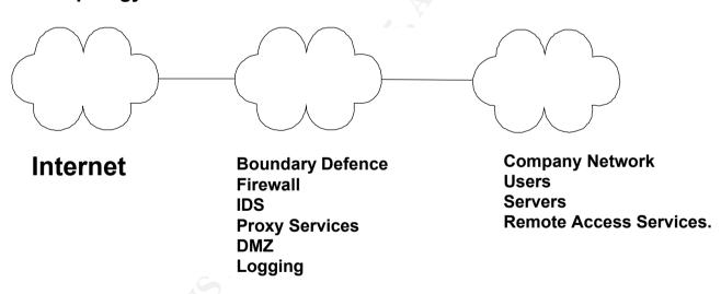
The old topology contains a good security between Internet and the Internal network. But there is limited "Defence in depth". The Internal Network grows and contains both users and servers. There is also a connection between the users and the Internet, rendering workstations and servers vulnerable to attacks direct from the Internet or by malicious software (virus or Trojan horses).
