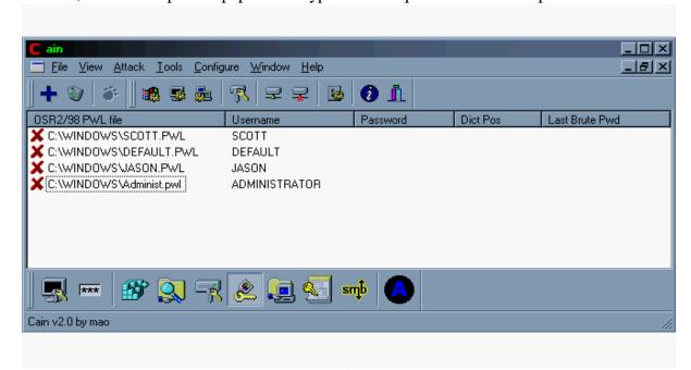
Note: Windows 9X uses the user logon name to generate the Encryption key. Therefore, you must know the user's login to be able to successfully decrypt a PWL file. Unfortunately the name of the PWL file is most often the login name.
