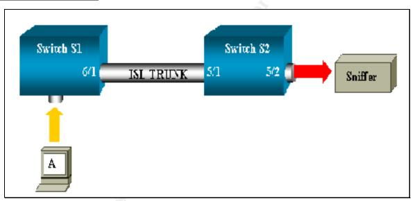
In this case, a user remotely monitors port 6/1 in swic h1 through port 5/2 in switch2. Two switches have a trunk port in between them.
