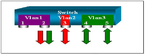
The above figure shows an example of monitoring multiple VLAN in a Catalyst Switch. Suppose a user wants to monitor VLAN2 and VLAN3 through port9/2. In this case, each SPAN belongs to a VSPAN since a port monitors multiple VLAN -based SPANs. To configure such case, a user can use the following command.
