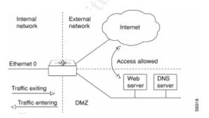
Assuming that CBAC is enabled on the router's internal interface (Ethernet 0) in the diagram, the operation of the context based access control would be as follows:
