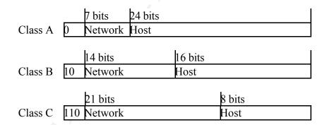
IPv4 network and host identifier in the IPv4 32 bit-addressing scheme
