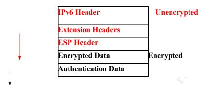
An encrypted packet using the ESP header
