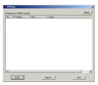
When you press the "scan" button a new creen will pop appear titled the scan arameters screen. On this screen please elect the IP Address button and enter 27.0.0.1. Other selectable items on this creen include the ability to scan by a ostname or a range of IP addresses. You lso have the option to Ignore the broadcast ddresses and what port you want to scan for
