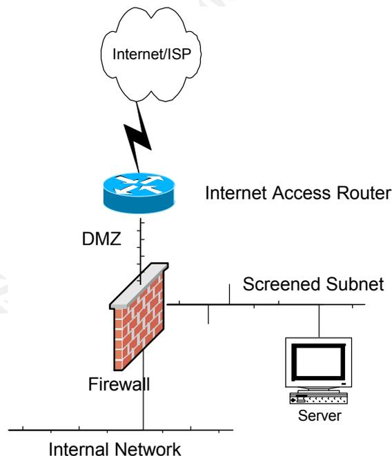
Most often, the connection to the ISP is some sort of serial line, but it can also be a high-speed line such as Ethernet or ATM. We will call this the outside interface of the router.
