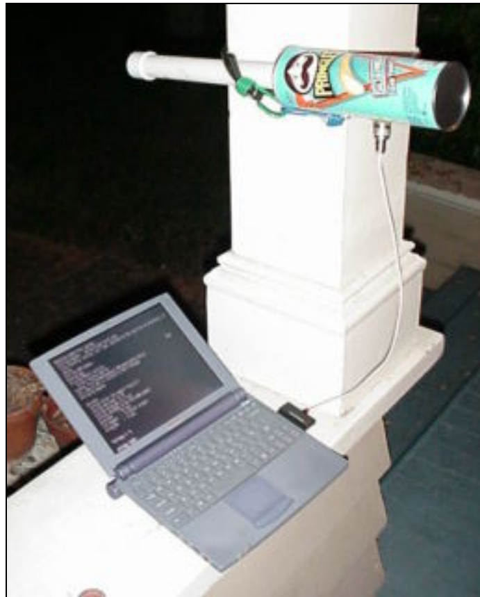
Pringles Antenna to scan Wireless LANS, source: [3]
