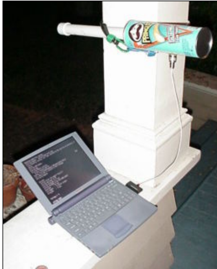
Pringles Antenna to scan Wireless LANS, source: [3]
