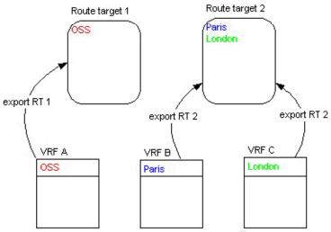
As a second step, VRF B imports Route Target 1. So does VRF C. After this step, both VRF B and VRF C know the required routing information to reach the OSS segment. However, they do not have any routing information on each other.
