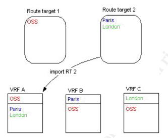
This topology is known as a hub and spoke, with the OSS VRF as a hub. The spokes can speak with the hub, but not between each other.
