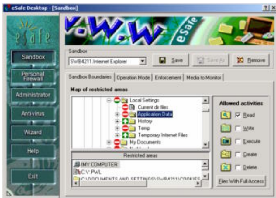
Graphical Interface showing ACL rule set for Internet Explorer
