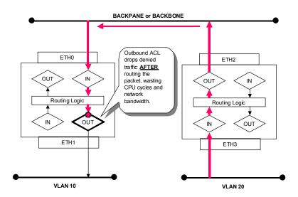
To provide the control desired, ACLs would need to be applied to ALL inbound interfaces on ALL routers connected to the company network. Although this is a desirable goal, there just was no practical way to accomplish such a feat in the time frame allotted and with the resources available. Consequently, we had to settle for applying ACLs to both the inbound and the outbound interfaces for the 10 VLANs remaining in our scope. Twenty ACLs were needed as shown in the table below:
