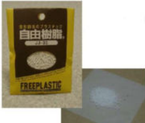
Fig. 2. Freeplastic used for fingerprint mold
