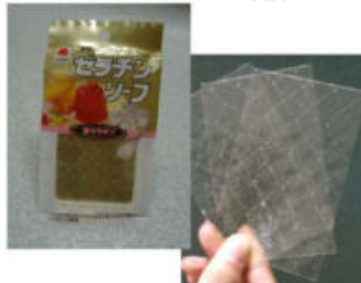
Fig. 3. Gelatin sheet used for gummy finger
