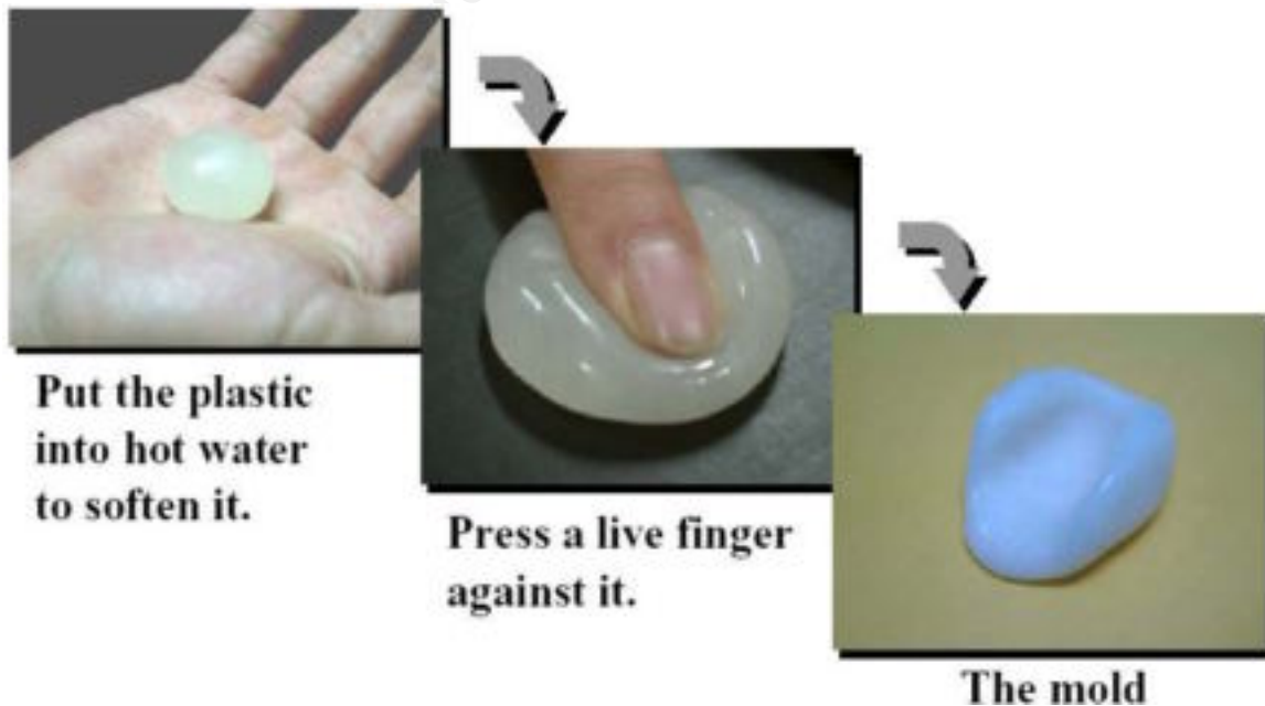
Fig. 4. Series of pictures demonstrating creation of fingerprint mold
