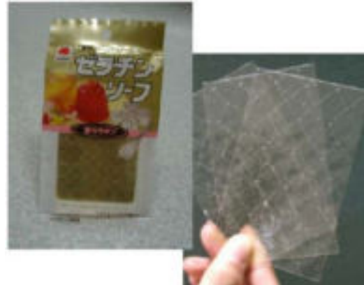
Fig. 3. Gelatin sheet used for gummy finger
