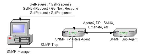
Figure 2. Flow of PDUs between SNMP managers and agents. Courtesy of iDefense (2)
