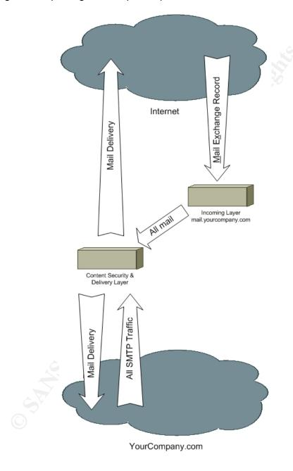
In this scenario we have one server handling the incoming layer and one server handling both content security and delivery layers. For this example, we are going to assume the content security layer is running a product that will use sendmail to deliver the filtered mail.
