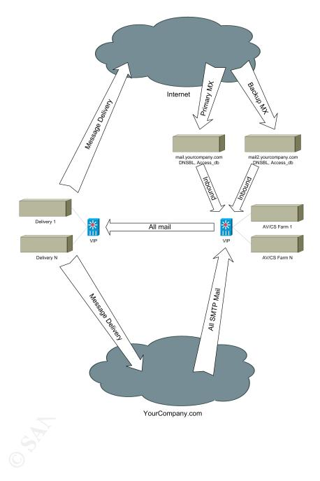
SECENERIO THREE: In this case all layers are separated and we have expanded the content security layer into two separate pieces to demonstrate how multiple content security vendors could be used together.
