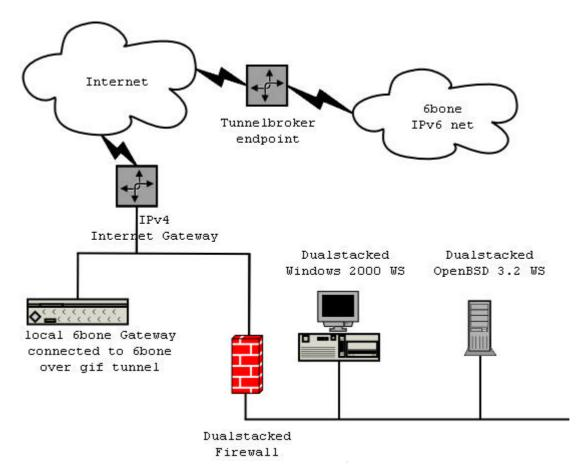
For IPv4 NAT/PAT will be used, for IPv6 routable addresses will be used, which is part of the real challenge of this setup.
