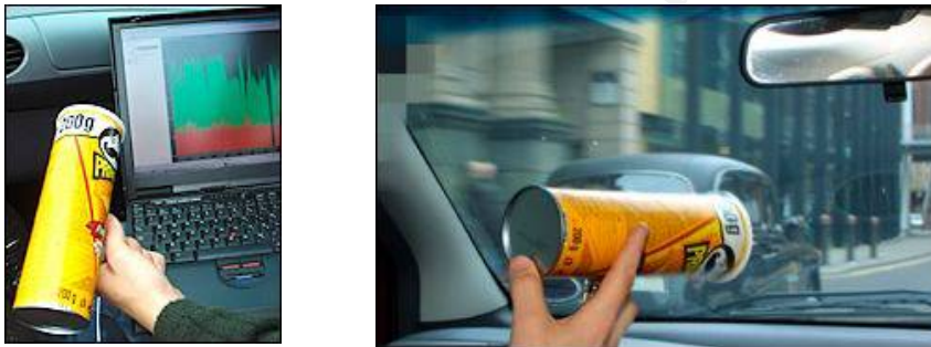
Figure 6 - Use of Pringles for Receiver
