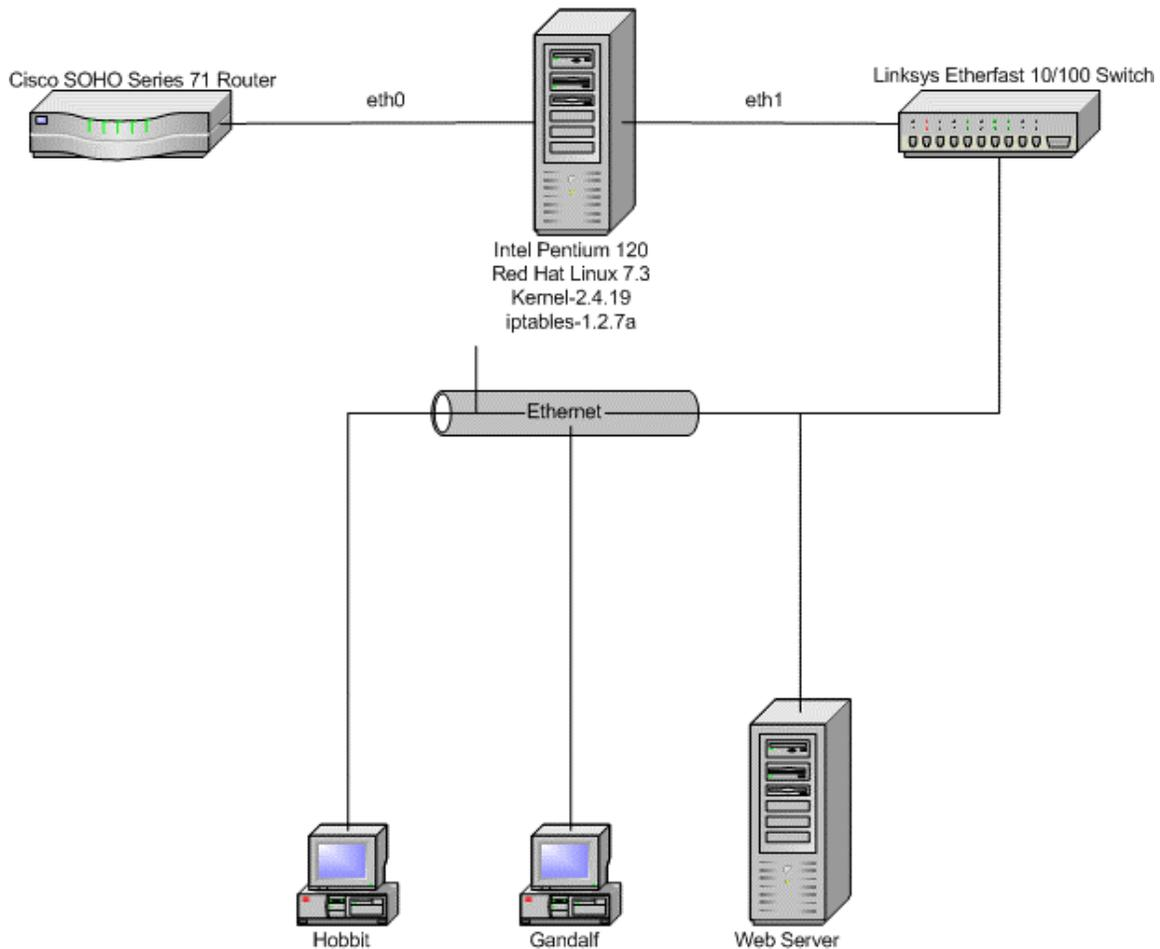
As you can see, a typical small office setup would consist of a router, a firewall, a switch, and finally, the related networked hardware attached to the switch.
