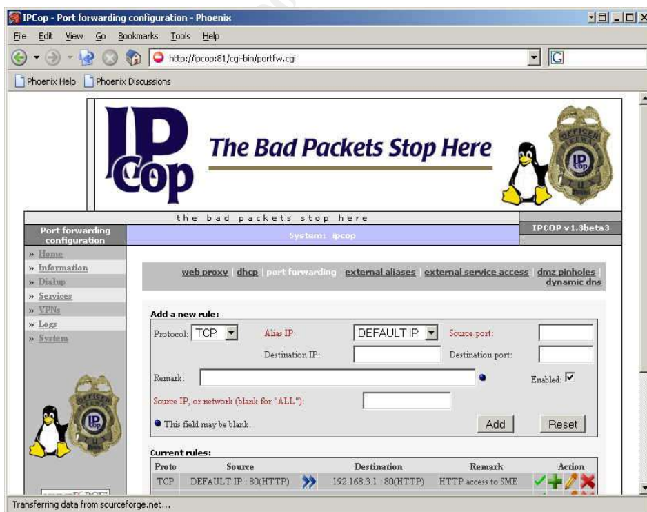
Illustration 5: firewall port forwarding configuration
