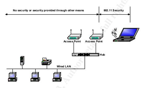
Wireless Security of 802.11 in a Typical Network
