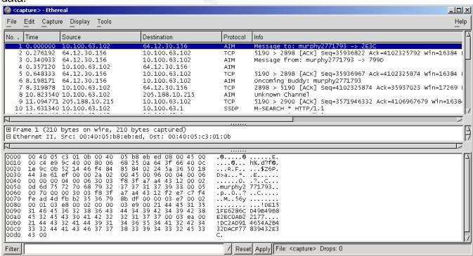
The response message is also encrypted. This case displays that when using Trillian client on both ends of an IM communication, that all data transmits as encrypted data.
