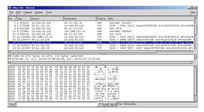
The response message is also sent in clear text without encryption. The data can not be encrypted if both users are not running the Trillian client application.
