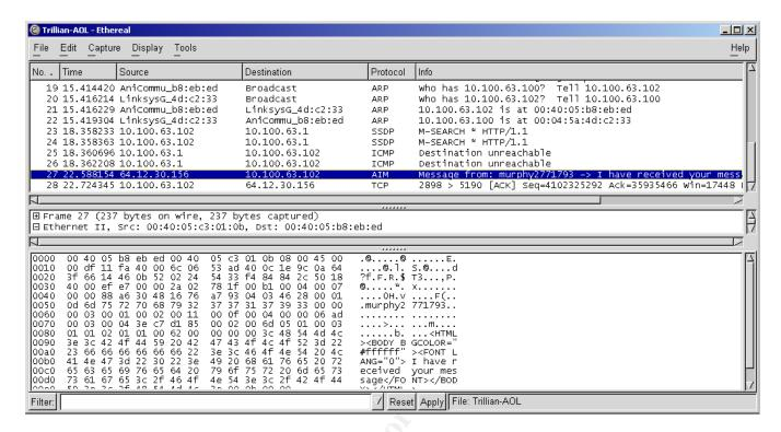
**Scenario 2:** This scenario examines AOL communications via one AOL client application and one Cerulean Studios' Trillian client application. The first screen print shows the data passed between the two users. Notice that even though Trillian is used, no feedback is given as far as establishing a Secure IM session. This is a result of not having both users running Trillian.
