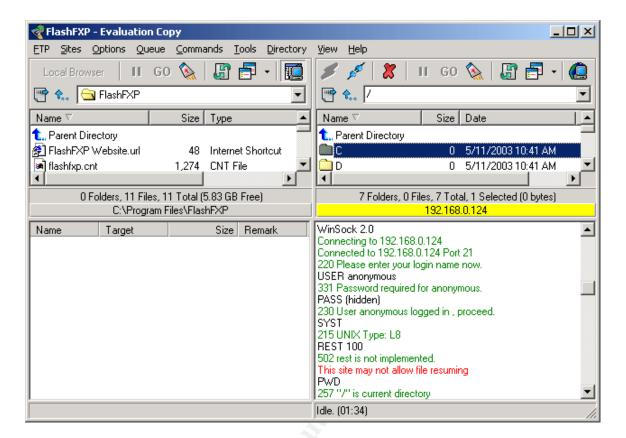
As shown in the screenshot, the FTP program was able to connect anonymously to the console. At this point, the connected FTP user has the ability to upload or download files, rename and even delete files off of the console's partitions.
