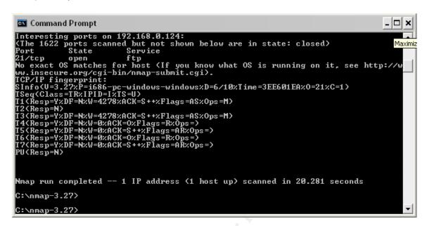
This scan attempts to identify the operating system. Notice that nmap was unable to determine the operating system, but notice the TCP/IP fingerprint that was returned.
