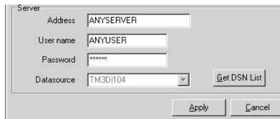
Figure 8. Example of a User Interface Configuration Exploit – Database Connection Parameters
