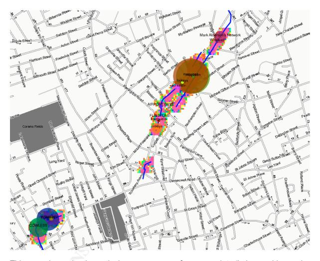
This map shows the theoretical coverage area of access points (in brown, blue and green), and also the interpolated real power levels as received on the WiFi monitor during the drive. This map was generated from Kismet results using the "gpsmap" program included with Kismet.
