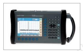
Spectrum analyzers are high-end devices that monitor the strength of various frequencies in the RF spectrum. Their use is not trivial, they are expensive and they need to be operated by qualified personnel. [willtek1]
