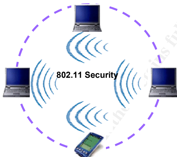
Figure 1 - 802.11 WLAN Implementation In Ad Hoc Topology
