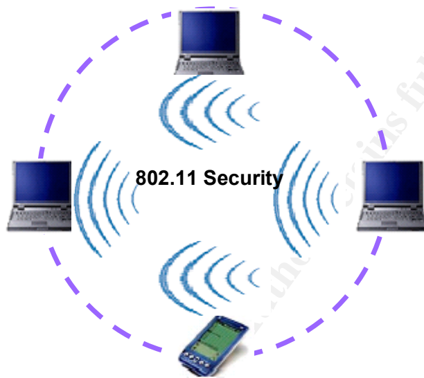
Figure 1 - 802.11 WLAN Implementation In Ad Hoc Topology
