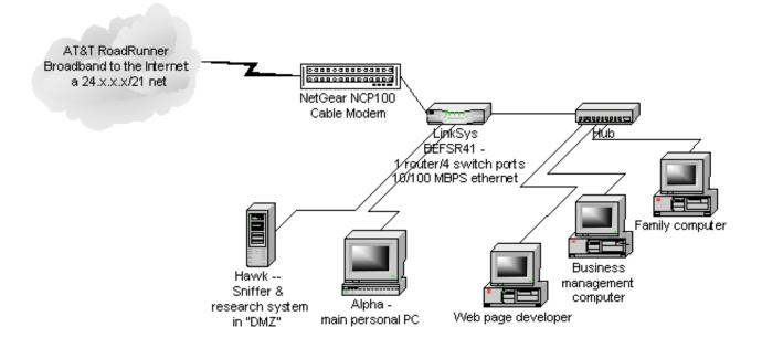
This diagram shows one possible arrangement to take advantage of the segregation available with a router. With all defaults in place (including no DMZ), the "Sniffer" box has almost nothing to watch. The combination of switching and routing, with a browser-based configuration GUI to set port options, reduces the network to external traffic specifically addressed - and by default returning from established connections only.
