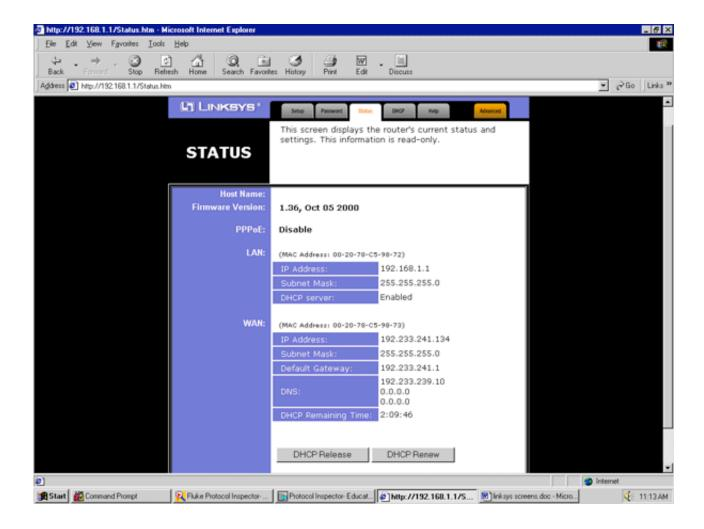
This is the Status screen after DHCP. The built in NAT function translates any traffic from the internal net destined for the world from the 192.168.x.x "private" to the "legal" external address obtained by DHCP. Simply stated, the external traffic from your systems all appear to be coming from a single, legal IP. This significantly reduces the intelligence gathering opportunities (net mapping) of most "hackers."
