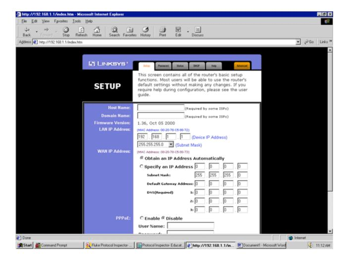
Opening setup screen. Note auto detect of MAC addresses and both DHCP & static IP options.
