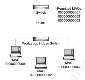
All of the mobile users have desks in an area serviced by the same workgroup switch. Each port permits the list of MAC addresses for each of the mobile users, as does the port on the backbone switch. Each mobile user can use any desk.
