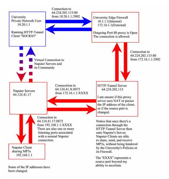
The two arrows between nodes represent a two way TCP connection.
