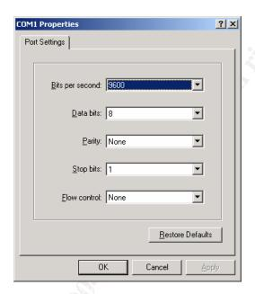
Connect the serial cable from your computer's serial interface (9 pins) to the PIX serial port. You may need to find a terminal adapter to go from 9-pin connector to RJ-45. Once everything is connected you can power on the PIX and you should be able to see IOS banner on your serial terminal.
