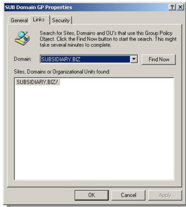
Figure 6: The Links tab of the Properties window on an example GPO. All sites, domains, or OUs to which the GPO is linked can be searched for and revealed here.
