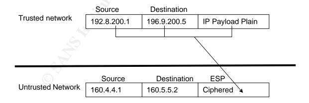
The idea behind tunnel is that the entire packet from a trusted network is encrypted and put in a new IP packet that has the address of a cipher system on another trusted network (and, if needed, the way to route the packet to this system). When the packet arrives at the remote end of the "tunnel", its contents is decrypted and the original packet is sent on the remote trusted network. When Tunnel Mode is used, hosts on trusted networks are hidden from hosts
