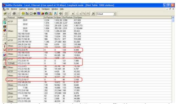
Again we can notice some hosts having outgoing traffic without getting any reply (no inbound traffic). This is seen on both HTTP (TCP port 80) and TCP port 445. Drilling down the conversations from these hosts for these protocols, here is what the traffic analyzer is reporting for HTTP traffic (TCP port 80):
