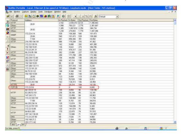
The host and protocol table shows a node with outbound packets, but no inbound at all, on TCP port 135. This should immediately attract attention. Filtering out from the capture the conversations from this host on that TCP port might be interesting. Here is the result of the filter:
