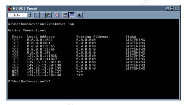
The above example is of a system with version 1.7 of NetBus running with the default configuration. One can see that ports TCP 12345 and 12346 are listening for connections.
