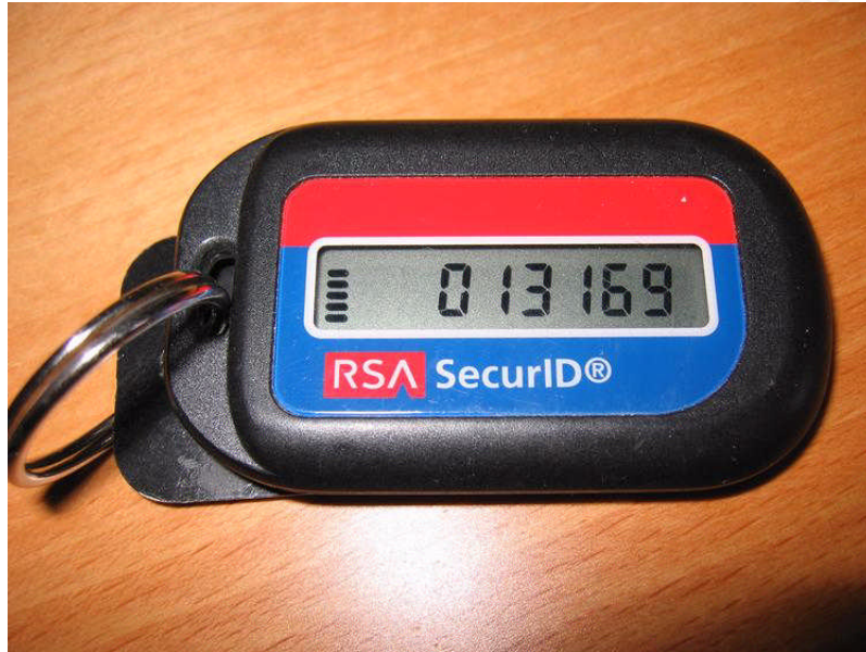
Figure 14-RSA SecurID for two factor authentication
