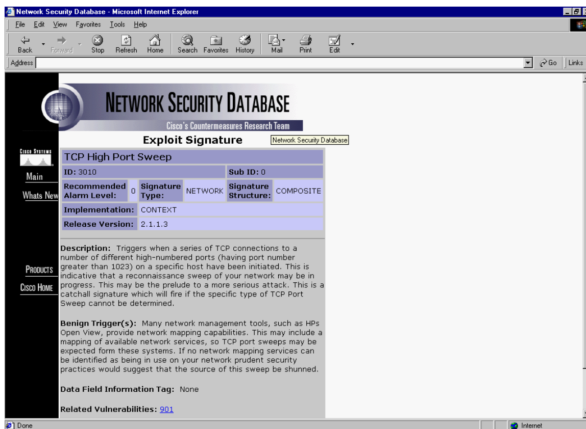
Figure 3. Cisco Network Security Database 3010 exploit signature for a TCP High Port Sweep.
