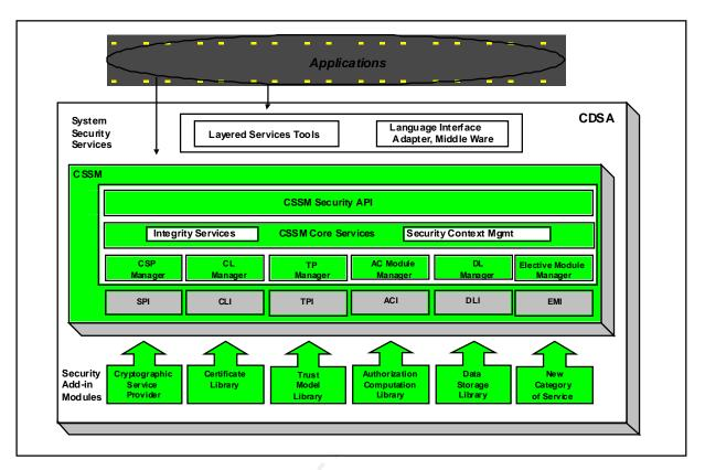
The diagram shows that CDSA is made up of three basic layers:
