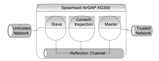
The slave board receives Internet requests from the untrusted network. The TCP headers are stripped off and the slave board maintains state with the Internet host. The slave board moves data to the reflective channel (out of band) where the data is written to both the content inspection board and the master board. The content inspection board checks
