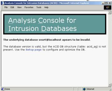
This is because ACID modifies the underlying Snort database table architecture. Click on the **Setup Page link** on the screen.
