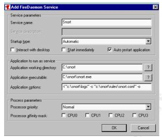
This will create an NT service called **FireDaemon Service: Snort** which will be set for automatic startup. Because you did not check the start immediately option the service will not be running. This is desired until we have all required pieces properly installed.
