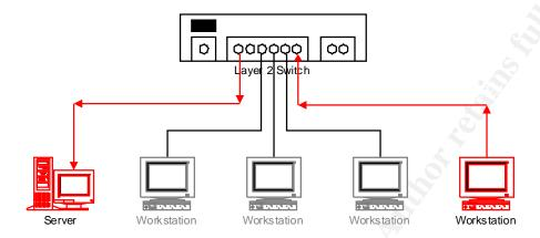
The computer sends the information to the switch, and the switch forwards the packet to the destination computer.
