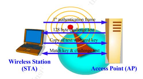
Figure 2: Graphical illustration of the shared key authentication process.
