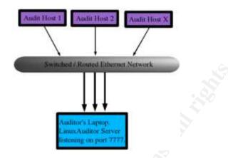
This graphic exemplifies how three audit hosts can write back to a single auditing machine and a single database. If desired, multiple audit hosts are able to write back to a single auditing machine running multiple database instances of the audit database. This type of configuration may be useful when the auditor desires to isolate subnets to a different audit database. The graphical configuration of such a setup is shown below.
