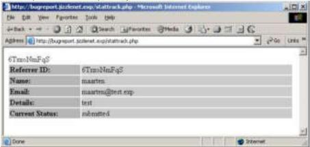
Inserting some random characters as a referrer id reveals nothing except the XSS flaw we already discovered. Inserting a quote or a semi -colon however, reveals the database we are dealing with as well as the real path of the document root.
